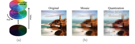
**Fig. 2.** An example of image mosaicing and quantization. (a) HSV cylinder is nonlinearly divided into small regions. (b) A high quality image along with its mosaiced image and quantized image by using quantization codebook provided by Fig. 2(a).
